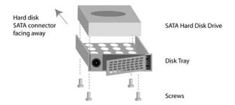
**4.** With the latch in the open position, slide the disk trays into the unit completely, securing the latch and closing the door.
